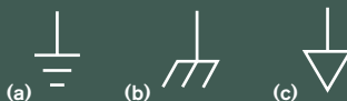
Figure A You should ensure the proper use of earth ground (a), chassis common (b), and signal common (c) for the grounds in your system.
